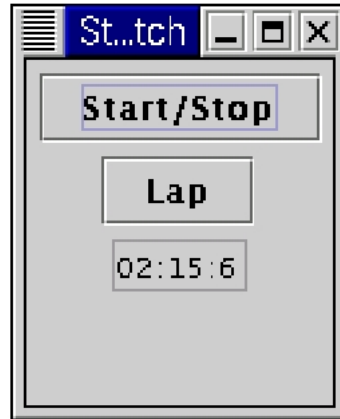
Figure 3.1: A simple graphical user interface for a two button stopwatch.
